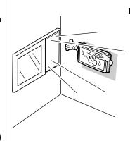
■ Do not install the unit in a location exposed to direct sunlight or strong light, as viewing the plasma display in an overly bright environment can be tiring for the eyes.
