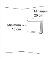
■ Do not block the ventilation holes, and be sure to leave sufficient space around the unit for ventilation.
